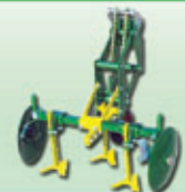
Elemento con dischi, 3 vomeri da 18 cm, supporto porta vomeri e ruota gomma Hoeing element with discs, 3 ploughshares of cm 18, ploughshare supports and rubber tyred wheel
