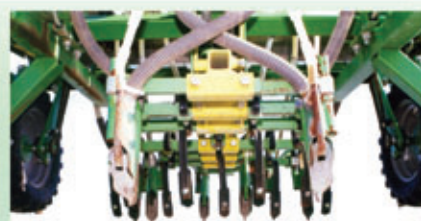
Assolcatori combinati molle vibranti e stivaletti Combined vibrant spring and coulters openers
